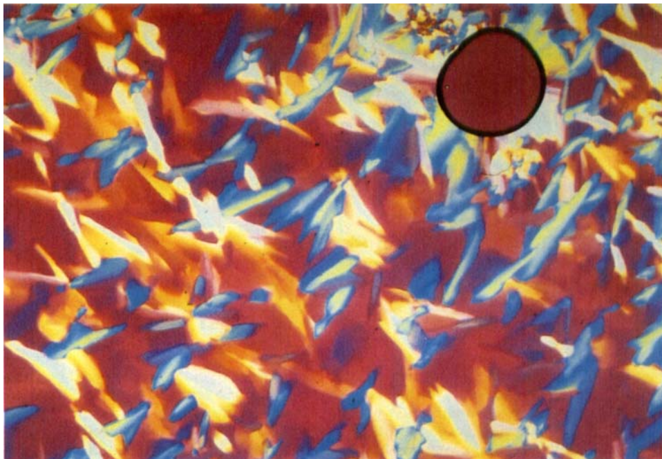
Figure 4. Optical texture of the freeze dried three chain diol with n=12 , between crossed polarizers after cooling from the isotropic melt, at 60^{\circ}\text{C} .
